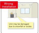
Use a stand to add sufficient height to protect the units heat exchanger from snow and prevent icicles forming during defrost operation.
